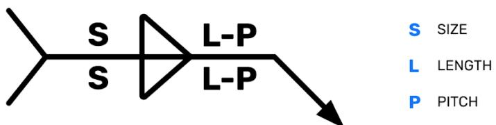
Fillet weld applications include continuous or intermittent conditions. Intermittent fillet welds can be specified as chain or staggered. A Stitch Weld is a common nonstandard term for intermittent welds.
