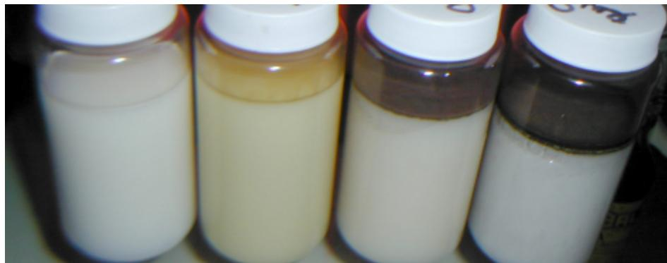
Clean coolant   Light Tramp Oil   Moderate Tramp Oil   Heavy Tramp Oil
