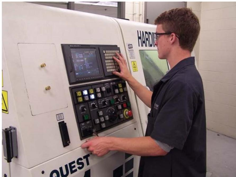
figure: An operator control panel mounted on the exterior of the machine control unit
