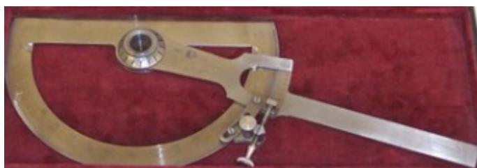
**Vernier bevel protractor**
