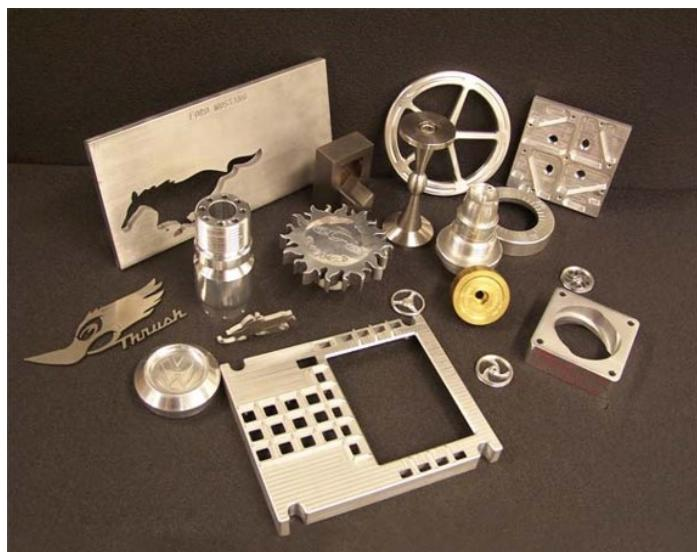
figure: Examples of some workpieces produced by CNC machines
