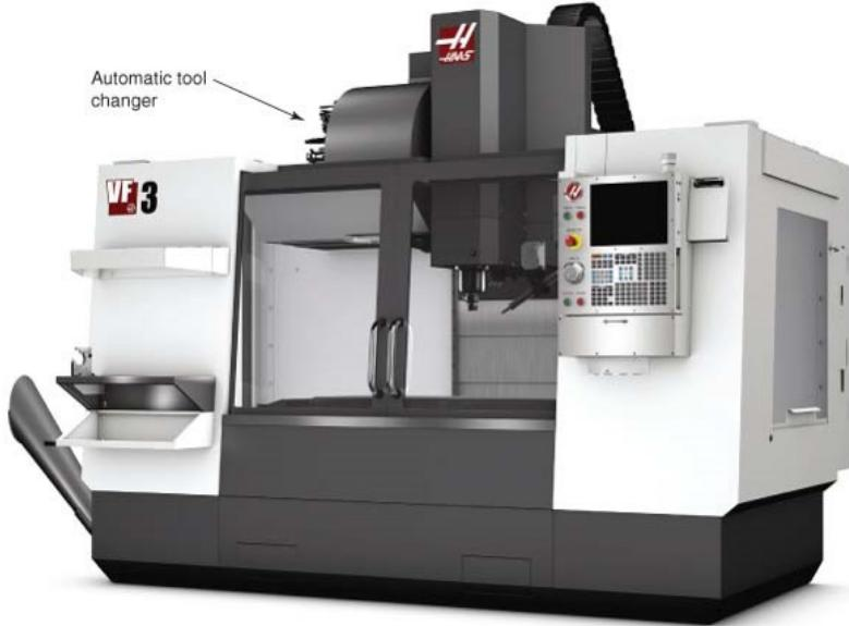
figure: A CNC machining center
