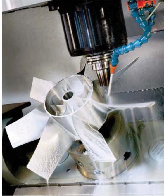
**CNC milling machines can produce complex part surfaces that would be virtually impossible to produce with manual milling machines**
