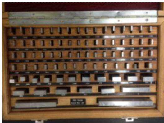
Many times, gage blocks are used on a flat reference surface such as a Surface Plate. Great care must be taken when handling and storing gage blocks. Any dirt or grit will impair their accuracy and reduce service life.
