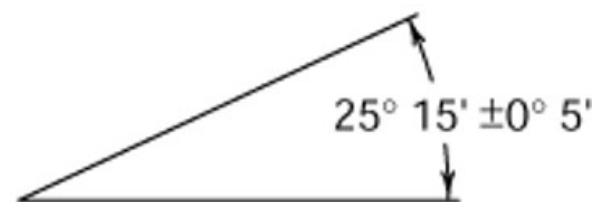
(B) Bilateral tolerancing
