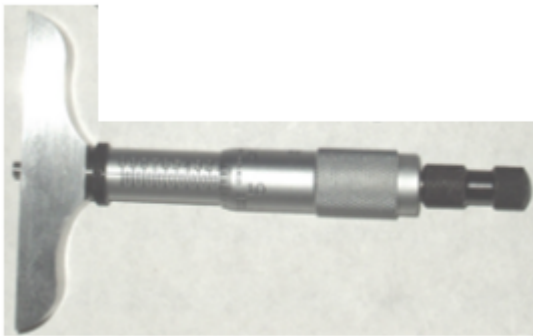
A depth micrometer with rods for different size ranges.
