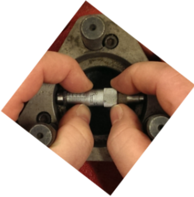
Taking a measurement using an inside micrometer.
